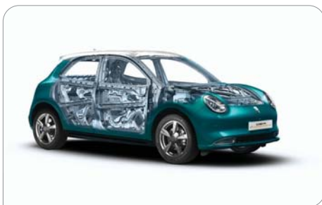
Iron Bone - Ultra-high Strength Steel Body Frame
