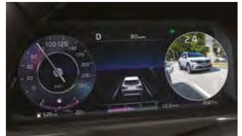
Fully Digital Supervision Cluster with Blind-spot View Monitor
